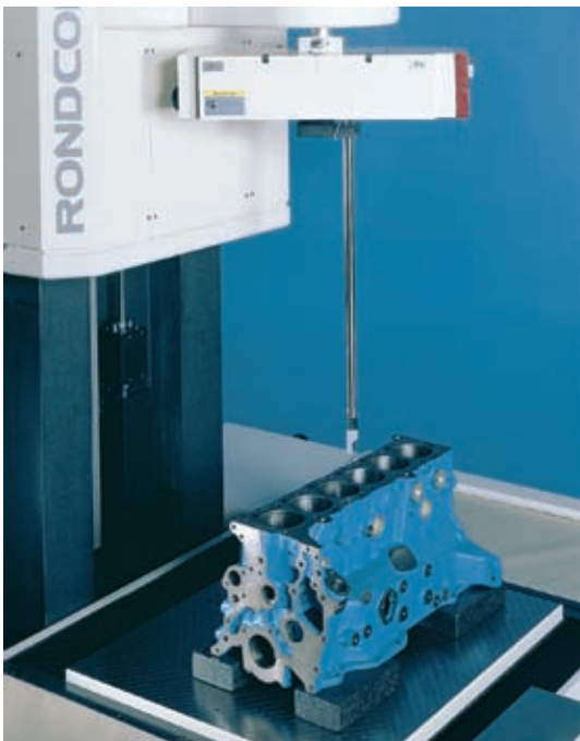
Typical applications for Rondcom 72/76: measurement of cylinder heads, engine blocks and crankshafts
